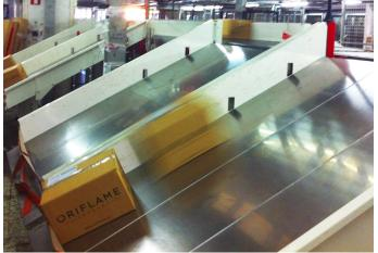
IT is controlled from the Kinematik Sorter Control Station. Signalling lamps with beepers located near the chutes are used to notify when a chute is full, increasing productivity.
