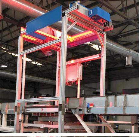
DWS system for measuring weight and dimensions, as well as save photos of items passing through.
